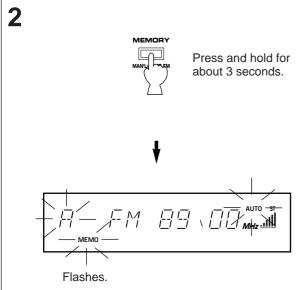
The automatic preset tuning begins from the frequency currently displayed. Received stations are programmed to A1, A2 ... A8 sequentially.
