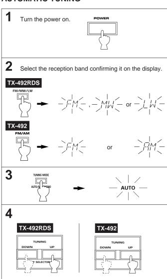
To tune to a higher frequency, press the UP button.
